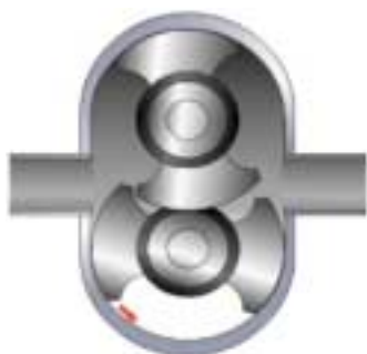
Fig. 1: With every degree of rotation, fluid displacement in the ECP pump is the same as the last and the next degree of rotation, resulting in a very smooth fluid flow. Since the body and rotor do not touch each other, there is no pump drag to overcome as with lobe and progressive cavity units.
